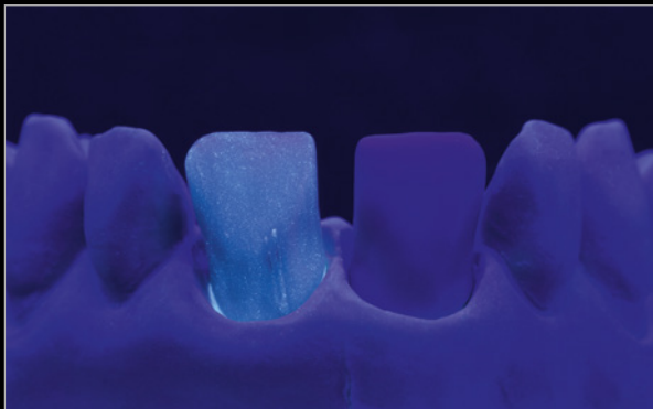
Fig 9 Image at tooth 21: Ideal fluorescence on a ceramic frame. Image at tooth 11: Zero fluorescence after none application of Adhesive 750
