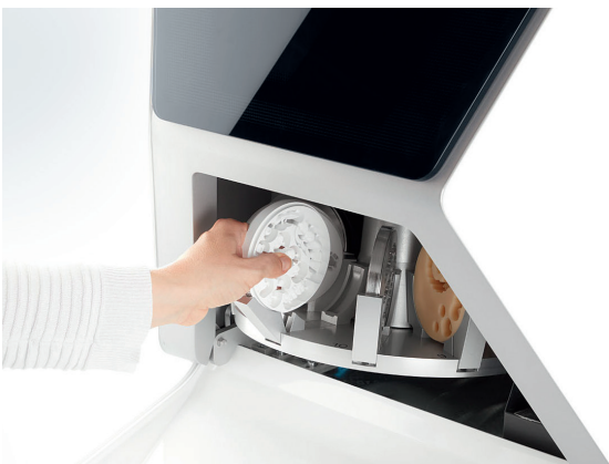
One-handed clamping made possible by DirectDisc Technology
